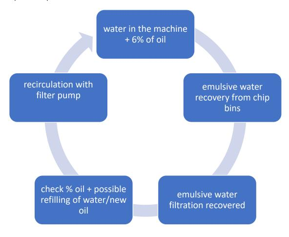
This system allows to recover 1,000 litres of emulsive water per week which saves us money by reducing the costs of disposal and purchase of oil. Above all, it allows to reduce both our annual water consumption (over 45,000 litres less) and the amount of chemicals delivered to the Company (about 3,000 litres less oil).
