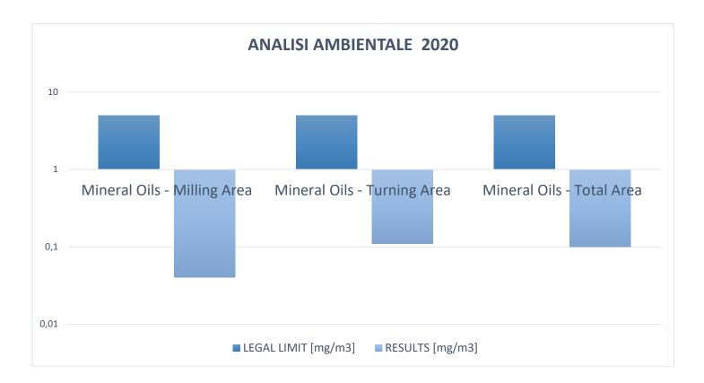
The graph clearly shows that the concentrations of agents harmful to the environment and to workers' health are significantly lower than the reference thresholds for the limit values provided for by current legislation.
